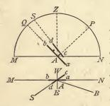
zenith, Q the celestial equator, and S the place of the sun at noon. Let A be the point where the instrument is set, which may be regarded as the center of the celestial sphere. Then the angle QAZ, or its equal PAN, is the latitude of the place of observation. The angle QAS is the declination of the sun, which is positive when
